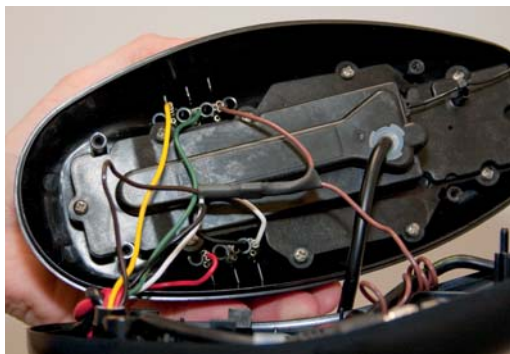
FIGURE 14 Insert AutoPilot wires into terminal holders.
